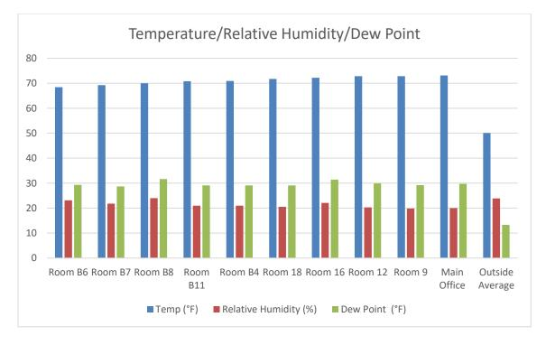
Temperature will affect the occupant's perception of IAQ based on employee comfort levels, effect of drafts or airflow, and humidity levels in a building. In most cases, simple adjustments to thermostats and direction of airflow from registers can improve perceived IAQ. As a reference, the temperatures recommended by ASHRAE for general office space ranges from approximately 68° to 75° Fahrenheit in the winter, and from approximately
